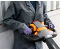
Pinch accident prevention switch
